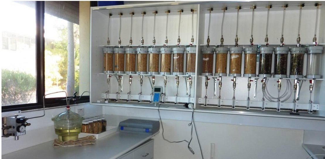
Figure 1. A gas purging flow system was used to treat the insects with constant concentrations of nitrogen and oxygen and maintained low carbon dioxide concentrations during the period of treatment. All 15 cylinders were filled with a known amount (1.8-2 kg) of grain (wheat, barley, oats, lupin and canola). A sealed sachet made of muslin cloth with 40-50 g of mixed age culture of stored grain insects with >200 adults were inserted at a depth of 6 and 23 cm.
