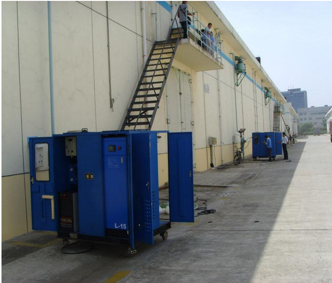
Figure 4. Commercial scale trials were conducted in Zhengding grain depot (38.145358,114.528351), China. Two units of 150 m 3 /hour membrane separation nitrogen generator were used to apply 99.5% purity of nitrogen to horizontal wheat storage (capacity of 10,000 tonne).
