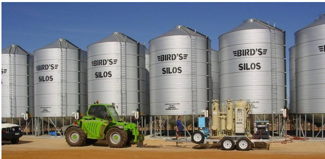
Figure 2. The farm bin-scale nitrogen application trials were conducted at Doug Clarke's farm near Lake Grace (33.117, 118.607), Western Australia. A pressure swing adsorption (PSA) nitrogen generator (capacity of 30 m 3 of 99.5% N 2 /hour) was used for purging nitrogen to wheat and canola bins (capacity of 75 tonne).
